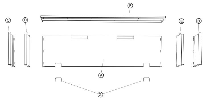
Insert (G) Gaskets into the two cutouts on the bottom edge of the (A) Back Panel, if not already installed.
