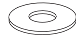
13. Washer \Phi 16 \times \Phi 6.5 \times 1 (4) Rondelle \Phi 16 \times \Phi 6.5 \times 1 (4) Arandela \Phi 16 \times \Phi 6.5 \times 1 (4)
