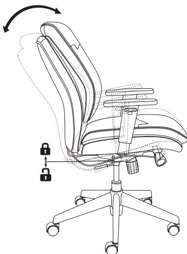
\*While seated, reach under the right side of the chair to find the height-adjustment handle. Pull the handle all the way out (away from the gas lift) to allow the chair to tilt backwards. To lock the chair in the upright or vertical position, sit upright and push the handle in towards the gas lift.
