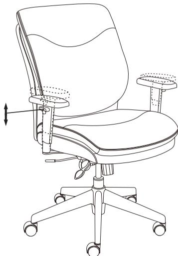
\*Pull up the buttons and hold to allow the arms to move up and down freely and then release the button once the desired height is reached.
