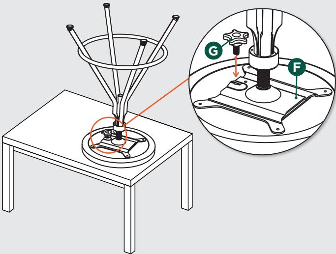
**2** Insert the shorter Black End of the Backrest Arm **D** into the opening of the Mounting Plate **F** until the Arm begins passing the Knob location. Tighten the Knob **G** securely at the desired horizontal location.
