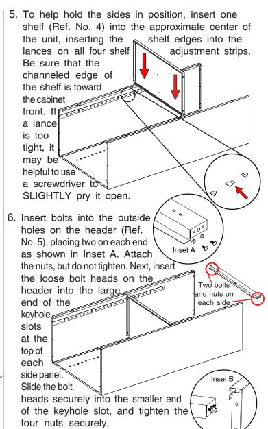
7. Attach the sill (Ref. No. 6) to the two holes on each side of the cabinet bottom, using the same technique you used to attach the header in step 6. Inset A Loosely place two bolts and nuts on each side, then Place bolt heads into slide into keyhole slots, slide to keyhole slots narrow end, and and secure. secure nuts
