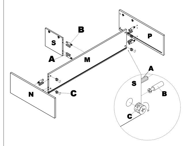
NOTE: The arrow on the face of the Cam (C) should point towards the Cam Post (B) for proper alignment.
